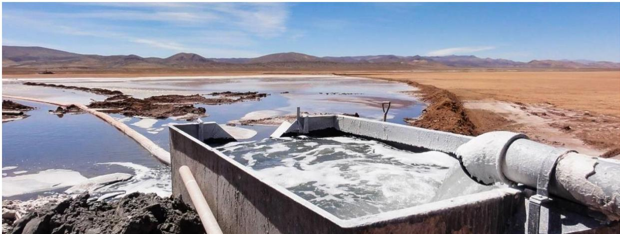
Figure 2: CAU07 wellhead configuration with flow meter showing the pumping rate for the 30 day constant rate pumping test
