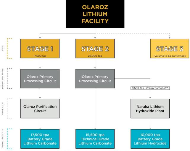
\* 9,500 tpa of Lithium Carbonate will convert to 10,000 tpa Lithium Hydroxide
