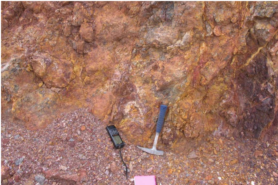
Marayes – high grade veining and altered country rocks with extensive goethite and limonite after sulphides
