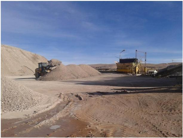
Crushed tincal ore being loaded into the feed bin.
