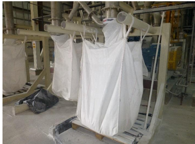
Bulk bags being filled with lithium carbonate to be sent to customers.
