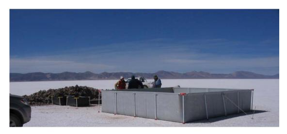
Larger scale batch processing test work has continued at facilities both at Olaroz and in Salta. The programme is nearly complete and will provide the process flow sheet and mass balance and for the scoping study currently being advanced.
